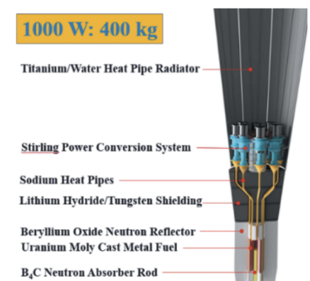
Fig. 1. Layout for 1-kW(electric) Kilopower system.
